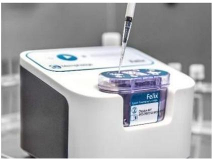
The Felix device consists of a console and single-use cartridges
